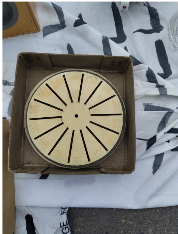
Slotted white viewing disc, seen from above. The radial slits function as the stroboscopic shutter that produces the illusion of movement.
