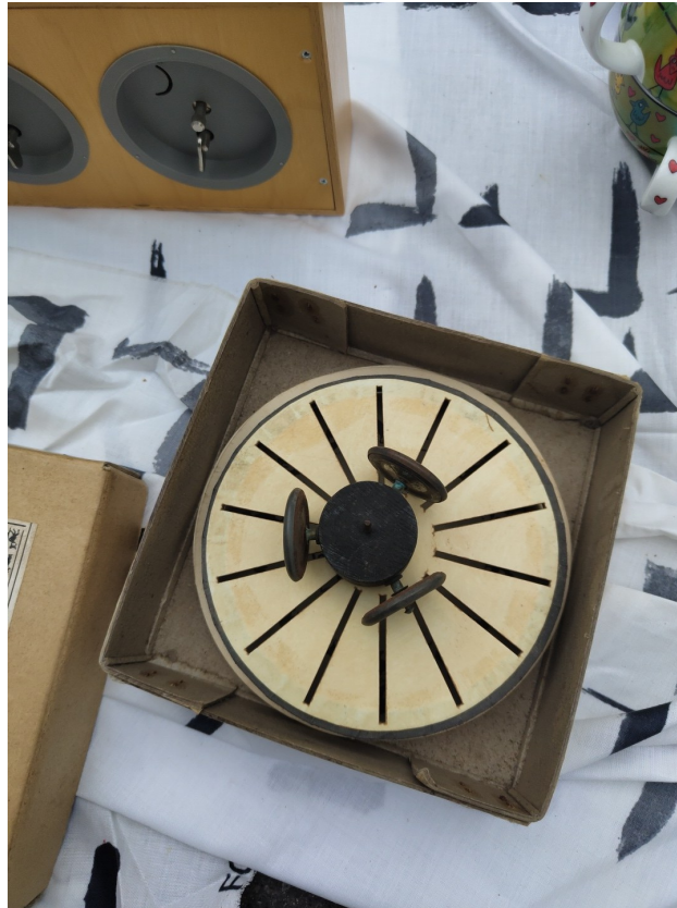
Slotted viewing disc with the central wooden carriage block and its three wheels in place – the rolling element that tracks the printed picture disc on the gramophone turntable.
