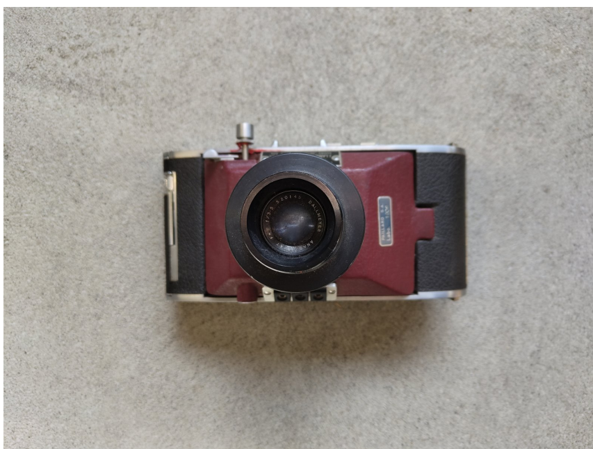
Fig. 1 — Top view, folded. The crimson-red body shell carries the Paillard SA laboratory inventory plate (left edge) and the Dallmeyer Oscillograph lens centred on the lens-board.
