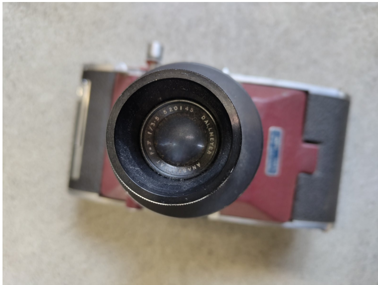
Fig. 3 — Dallmeyer Anastigmat lens engraving (axially recessed in helical tube). Marking: DALLMEYER ANASTIGMAT F=3 f/3.5 520145.
