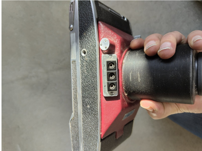
Fig. 4 — Right body flank: three coaxial synchronisation sockets (B / C / M) and helical focusing barrel of the Dallmeyer objective.
