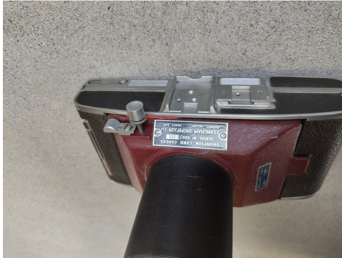
Fig. 2 — Maker's plaque on the top deck. The serial scheme 400/xxx indicates model variant 400, production number 225. A related machine (N° 410/107) is preserved in the Science Museum Group collection, London.
